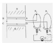
**Working:** When the coil is made to rotate in clockwise direction, the magnetic field linked with the coil changes. This induces an electric current in the coil ABCD. During the first half of the rotation, the current flows along ABCD  $R_1$   $B_1B_2$ . During the second half of the rotation current is induced in the coil along DCBA  $R_2$   $B_2$   $B_1$ .
